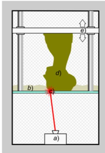
**Figure 3: Schematic representation of Stereolithography [3]**
