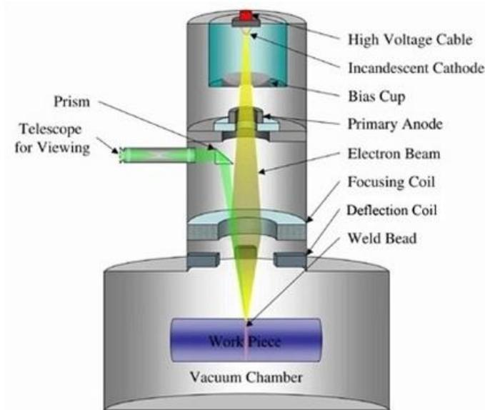
**Figure 5: Schematic representation of EBM**
