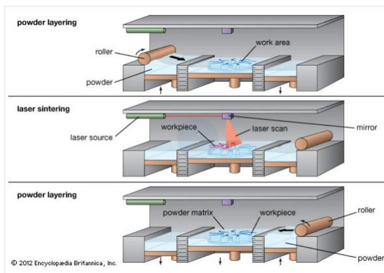
**Figure 1: Selective Laser Sintering scheme**
