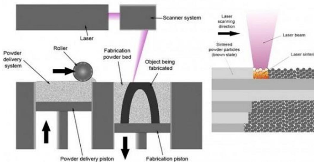
**Figure 2: Selective Laser Melting scheme**
