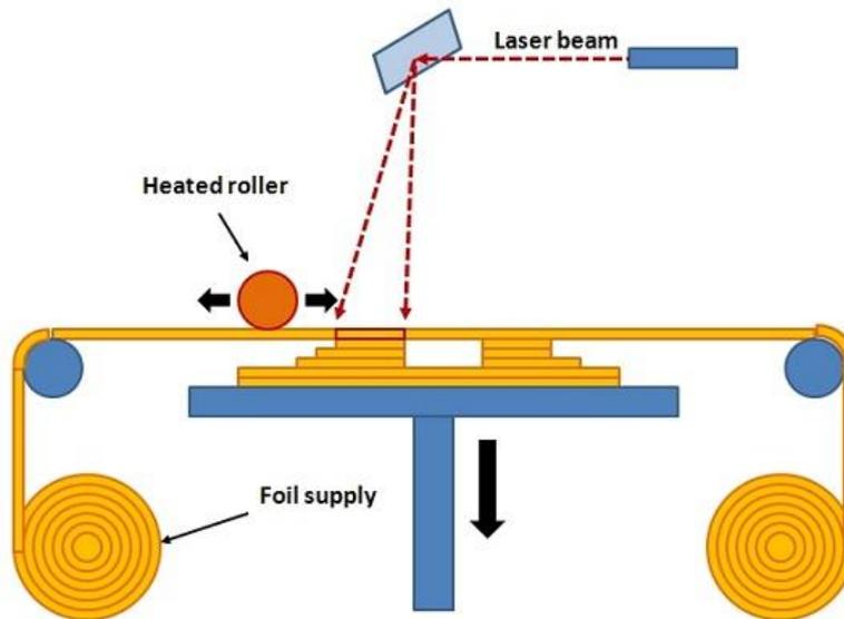
Figure 6: Schematic representation of LOM
